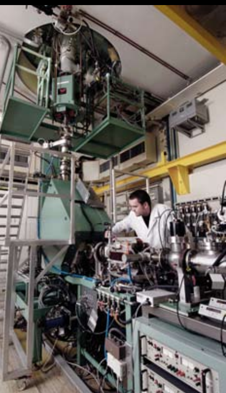
Analysing magnet at the Van de Graaff accelerator (2007). The precise energy of the ion beam is defined by the analysing magnet (centre of photo) and a pair of slits, which regulate the accelerator high-voltage terminal to give a beam energy precision of about 0.2%.
