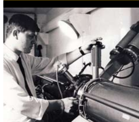
Adjusting the coils at a section of the linear accelerator. On the right-hand side is the connection to the klystrons.
