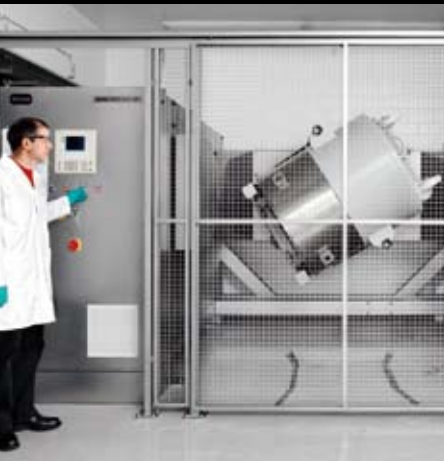
Facility for large-scale mixing of powders (up to 550 litres or 400 kg) during reference material production (2008).
