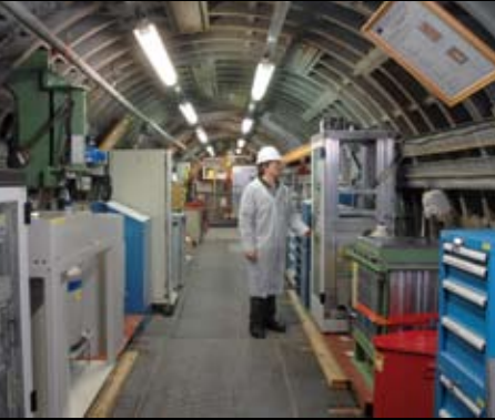
Underground laboratory for the ultra-low-level gamma-ray spectrometry. The background radiation is 10,000 lower than above ground.
