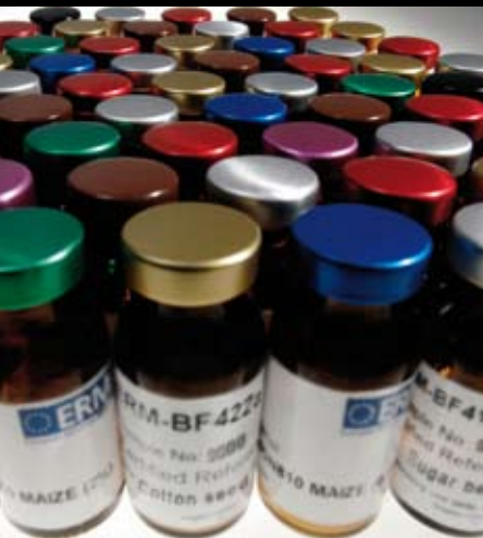
Reference materials for genetically modified organisms. IRMM was the first European reference material producer to obtain accreditation according to ISO Guide 34.
