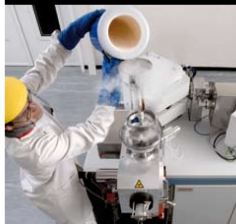
Liquid nitrogen is poured into a state-of-the-art mass spectrometer used to measure plutonium isotope ratios (2008).
