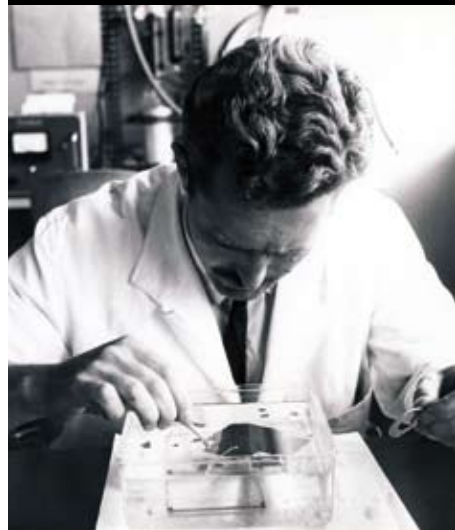
A thin carbon foil is carefully removed from the surface of the water.
